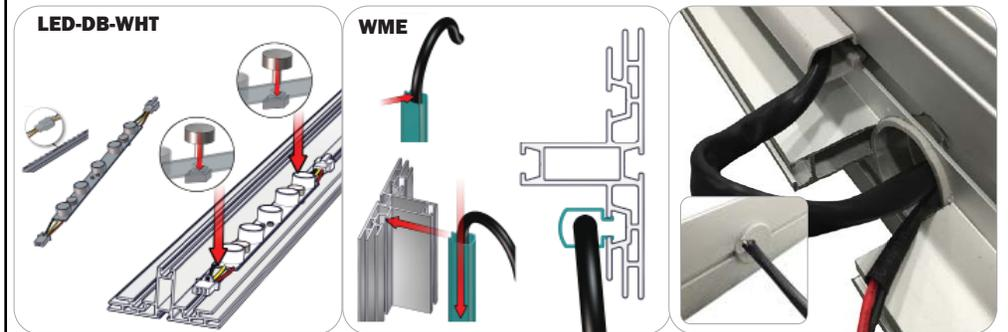
Be sure to fully assemble all frames before using the internal lighting components. With the thumbscrews loosened, place the light strips on the frame, then hand tighten them in series, male to female connections with extension cords. Do not over tighten the thumbscrews. Snap on the wire management extrusions with the power cord extensions in place. Reference the Internal Lighting Diagram for more details.
