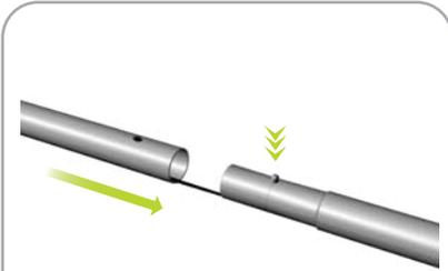
Connect bungee tubes by lining up holes with snap buttons
